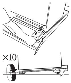
Make sure you lower BOTH REAR ROLLERS. There are two adjusting nuts, one for each roller, at both the front bottom corners of the range.
